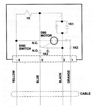
Fig. 10: D80D General Wiring Diagram
